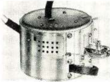
Fig. 3. The completely shielded tuner assembly of the Regency converter.
