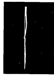
7F7 Hor. Preseparator, AGC Rect. & Vert. Preseparator. Cathode of AGC Rect. & Hor. Presep. (Test Point 5) 0.5 Volts P to P. (Vertical)
