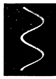
6AL5 AFC Disc. Diode Plate to Diode Plate (Test Point 10 to Test Point 11). Ground Lead of Oscilloscope to Pin 7 8 Volts P to P. (Horizontal)
