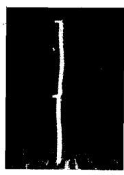
7F7 Hor. Preseparator, AGC Rect. & Vert. Preseparator. Cathode of AGC Rect. & Hor. Presep. (Test Point 4) 1.5 Volts P to P. (Vertical)
