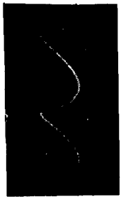
6B6G Hor. Output. Cathode (Test Point 15) 15 Volts P to P. (Horizontal)
