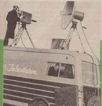
The mobile unit of the Television station is actually a complete transmitting station. The picture is relayed to the main transmitter where it is rebroadcast. Notice the disk-like relay transmitting antenna.
