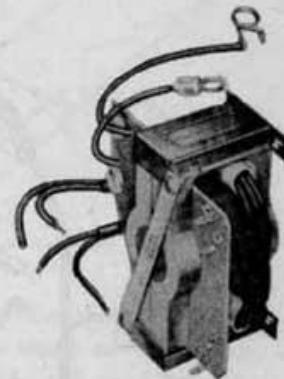
11T5 Horizontal Deflection Output and High Voltage Transformer
