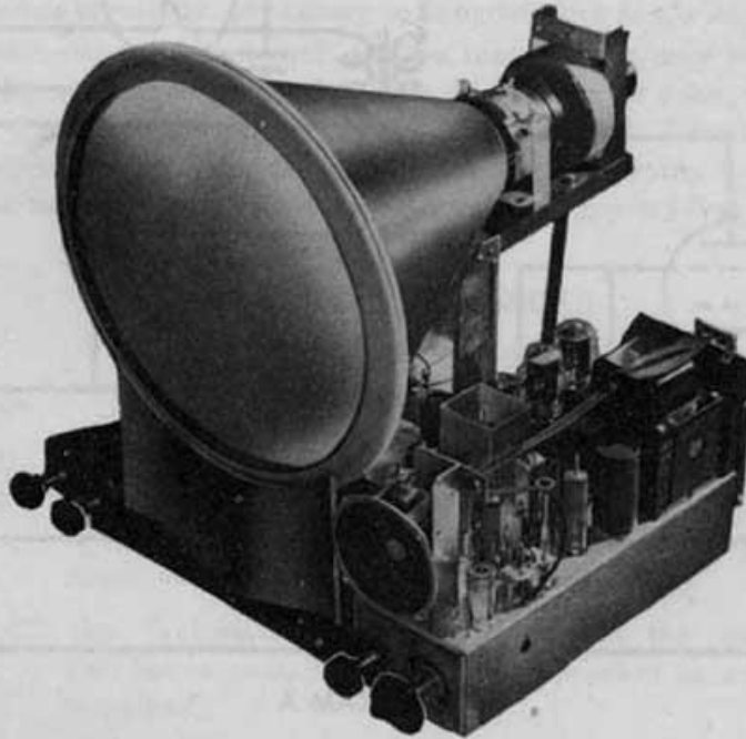
Tech-Master 630-TK Chassis With 16AP4 Kinescope Using Tech-Master Universal Adjustable Brackets 16AP4 is shown with plastic mounting ring and sleeve.
