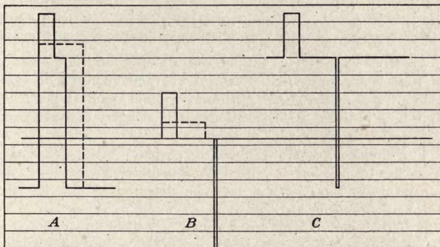
FIG. 24.—(A) Video signal corresponding to an all-white picture. (B) Signal for an all-black picture, except for a small white area. (C) Same as (B) except that d-c transmission is employed. (R. D. Kell.)
