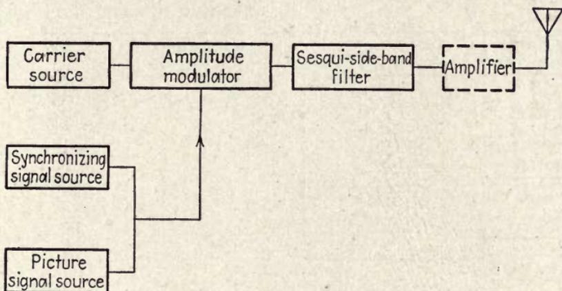
FIG. 73.—Arrangement of transmitter components for R.M.A. standard signal.
