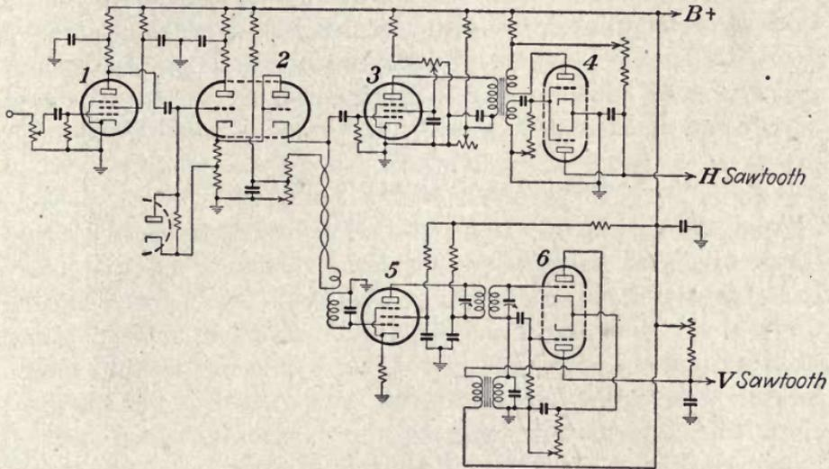
FIG. 87.—Pulse separator circuit. (Campbell and Lempert.)
