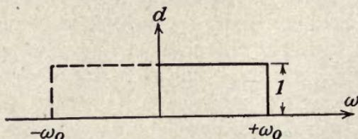
FIG. 31.—The admittance characteristics,  $d$  vs.  $\omega$ , of a flat passband filter, with unity admittance within the passband. The phase characteristic,  $\phi(\omega) = k\omega$ , is uniform within the same limits.
