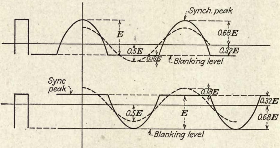
Fig. 79.—Detail of the 500-ke vertical pulse. (A. V. Bedford and T. T. Goldsmith, Jr.)
