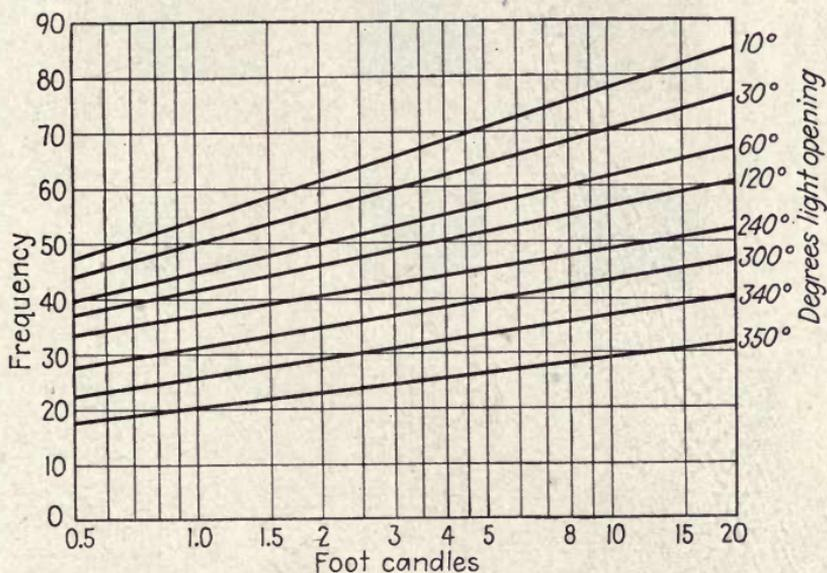
Fig. 54.—Conditions for just-noticeable flicker, with sector disk test, taken from E. W. Engstrom. (A. V. Bedford.)
