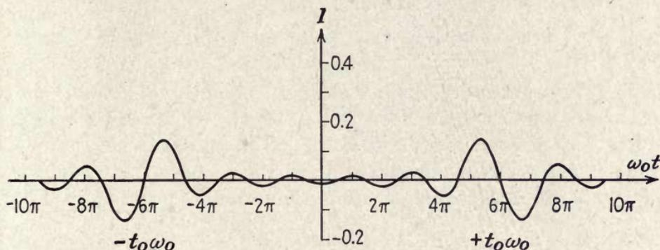
FIG. 40.—Response of the filter of Fig. 39 to the square pulse, for  $c = 0$ , and  $\phi = 0$ . The peak-to-peak amplitude is 0.275. The gain in signal to noise at the top frequency is 12.5 db, whereas the loss at zero frequency is infinite.
