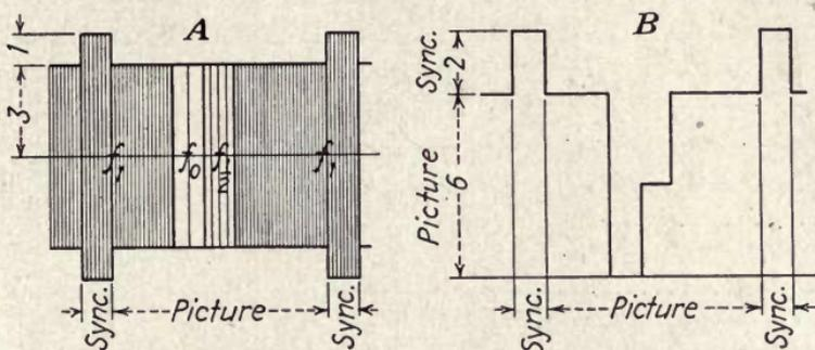
FIG. 70.—Transmitter-output waveforms, method 5. (R. D. Kell.)
