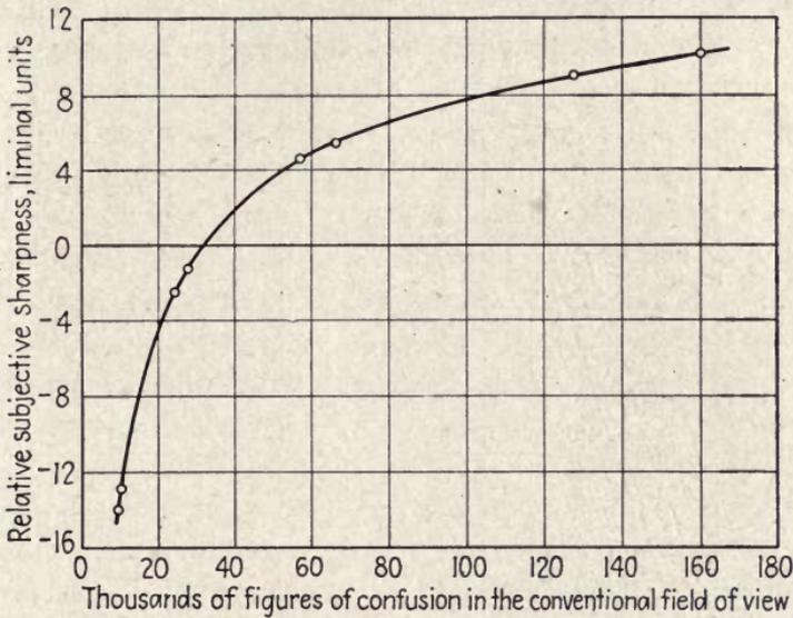
FIG. 61.—Sharpness of motion pictures as a function of resolution. The conventional field of view is a rectangle whose height is  $\frac{1}{4}$  the viewing distance and whose width is  $\frac{4}{3}$  the height. Reference sharpness is approximately that of a 240-line, 24-frame per second, 806-kc television image. Curve based on 270 observations at a viewing distance of 30 in. (*M. W. Baldwin, Jr.*)
