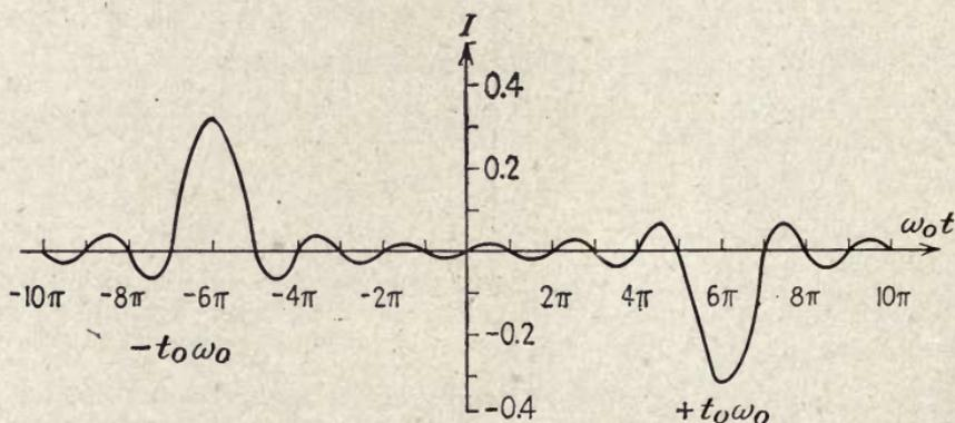
FIG. 38.—Response of the filter of Fig. 34 to the square pulse, for  $c = 0$  and  $\phi = \pi/2$ . The peak-to-peak amplitude is 0.635. The gain in signal to noise at the top frequency is 5 db, but the loss at zero frequency is infinite.
