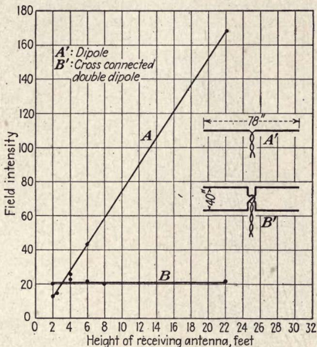
FIG. 102.—Field intensities as a function of height. Receiving antenna rods horizontal and oriented broadside to transmitter; transmitter loop horizontal,  $2\frac{1}{2}$  ft. above ground and 100 ft. from receiving antenna. (W. L. Carlson.)
