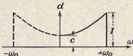
FIG. 39.—Admittance characteristic of a predistorting filter with admittance increasing as the square of the frequency, from admittance  $d = c$  at zero frequency to unity at the top frequency. Phase characteristic  $\phi(\omega) = k\omega$ .
