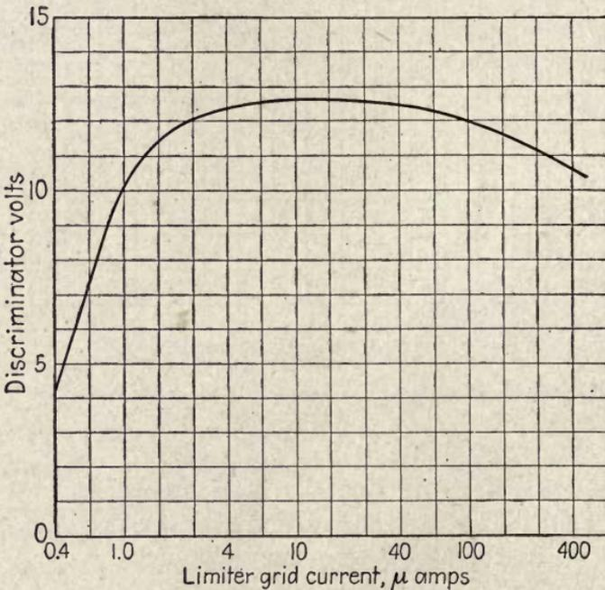
FIG. 16.—Limiter characteristic, taken at 2,859 kc. (center frequency 2,900 kc.),
