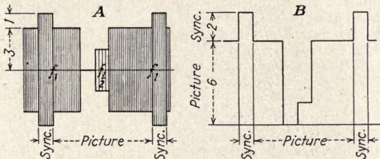
FIG. 71.—Transmitter-output waveforms, method 6. (R. D. Kell.)
