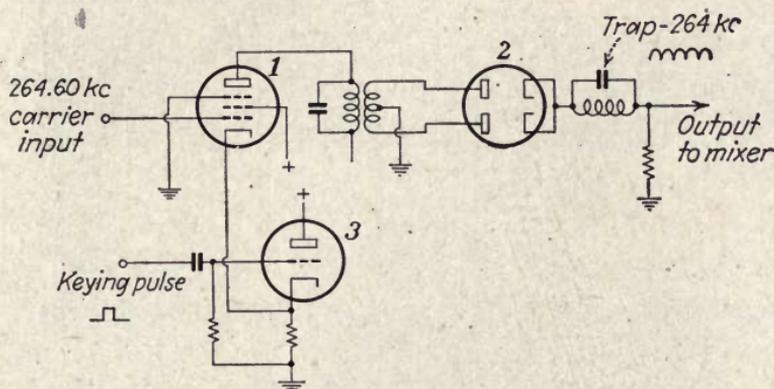
FIG. 82.—Full-wave rectified carrier circuit for vertical synchronizing pulse wave
