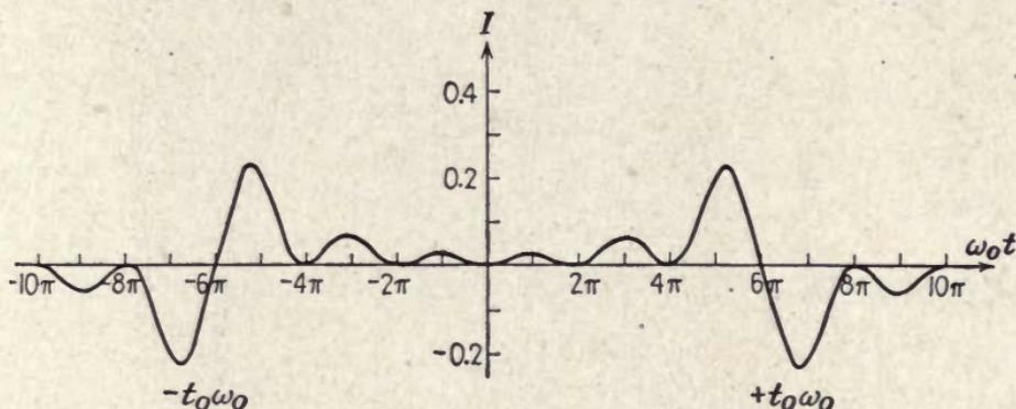
FIG. 35.—Response of the filter of Fig. 34 to the square pulse, for  $c = 0$  and  $\phi = 0$ . The peak-to-peak amplitude is 0.465. The gain in signal to noise at the top frequency is 8 db, but the loss at zero frequency is infinite.
