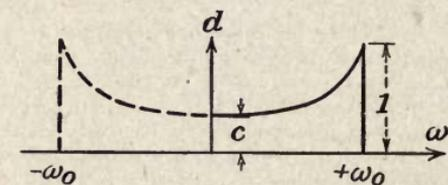
FIG. 42.—Admittance characteristics of a predistorting filter with admittance increasing as the cube of the frequency from  $d = c$  at the zero frequency to unity at the top frequency. Phase characteristic  $\phi(\omega) = k\omega$ .
