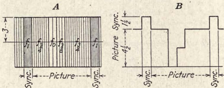
FIG. 67.—Transmitter-output waveforms, method 2. (R. D. Kell.)
