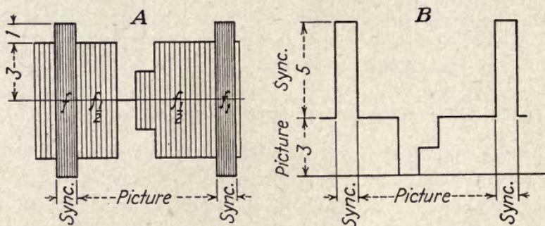
FIG. 69.—Transmitter-output waveforms, method 4. (R. D. Kell.)
