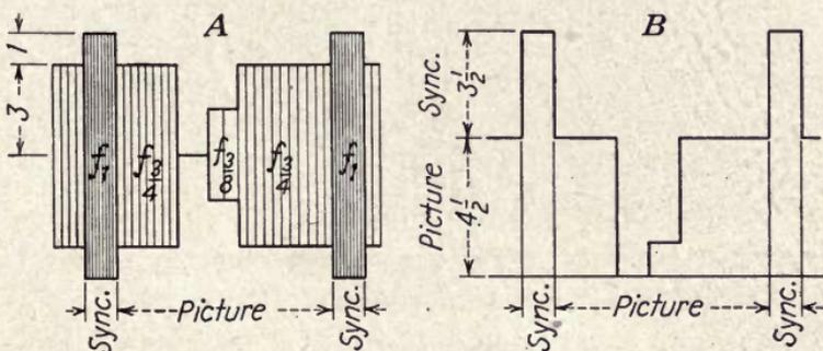
FIG. 72.—Transmitter-output waveforms, method 7. (R. D. Kell.)
