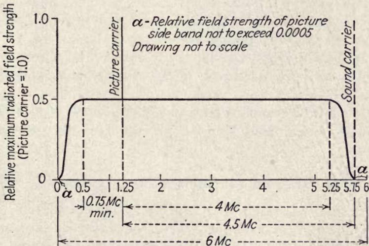
FIG. 1.—Idealized picture transmission amplitude characteristic.
