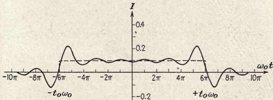
FIG. 41.—Response of the filter of Fig. 39 to the square pulse, for  $c = 0.1$  and  $\phi = 0$ . The peak-to-peak amplitude is 0.34. The gain in signal to noise at the top frequency is 11 db, whereas the loss at zero frequency is 9 db.
