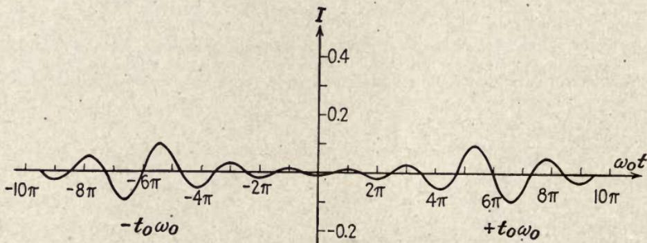
FIG. 43.—Response of the filter of Fig. 42 to the square pulse, for  $c = 0$  and  $\phi = 0$ . Peak-to-peak amplitude 0.2. Gain in signal to noise at top frequency is 15.5 db; loss at zero frequency is infinite.
