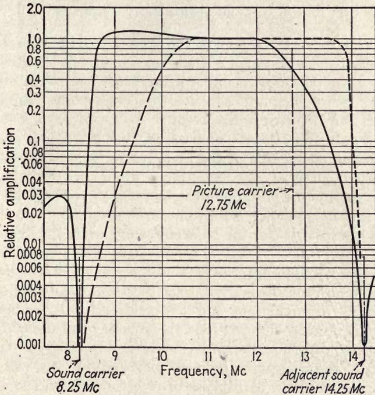
FIG. 28.—Picture amplifier characteristic. (R. D. Kell.)
