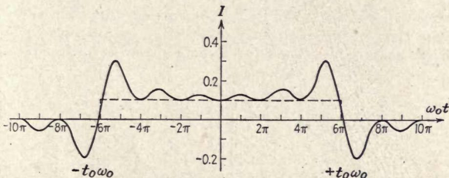
FIG. 36.—Response of the filter of Fig. 34 to the square pulse, with  $c = 0.1$  and  $\phi = 0$ . The peak-to-peak amplitude is 0.5. The gain in signal to noise at the top frequency is 7.5 db, the loss at zero frequency 12.5 db.
