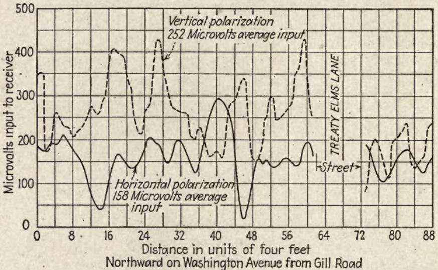
FIG. 105.—Variation of signal strength with distance, 69 Mc, comparing vertical with horizontal polarization. (W. L. Carlson.)
