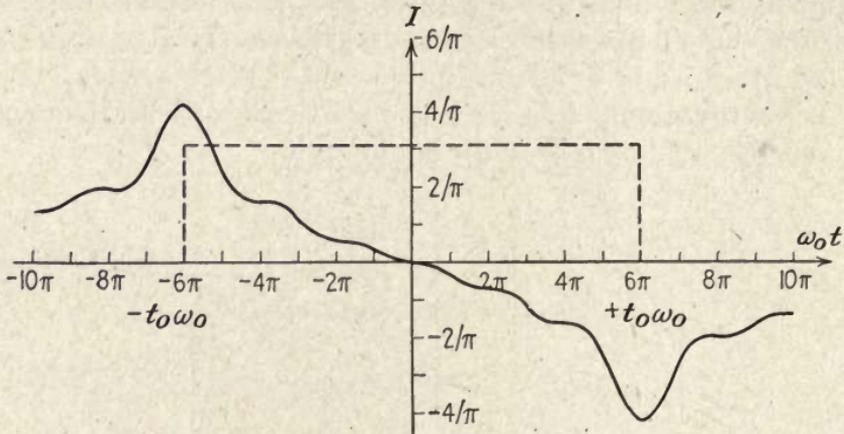
FIG. 33.—The response of the flat filter to the square pulse, when the filter phase characteristic is  $\phi(\omega) = \pi/2$ . The peak-to-peak amplitude is thereby increased to 2.68. The loss in signal to noise at the low frequencies is 7 db, at the top video frequency 7 db.
