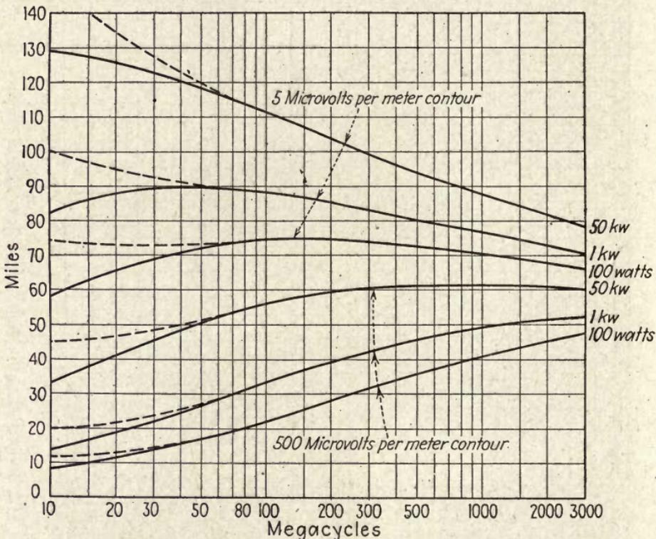
FIG. 115.—Signal range for high-frequency broadcast stations (IV).
