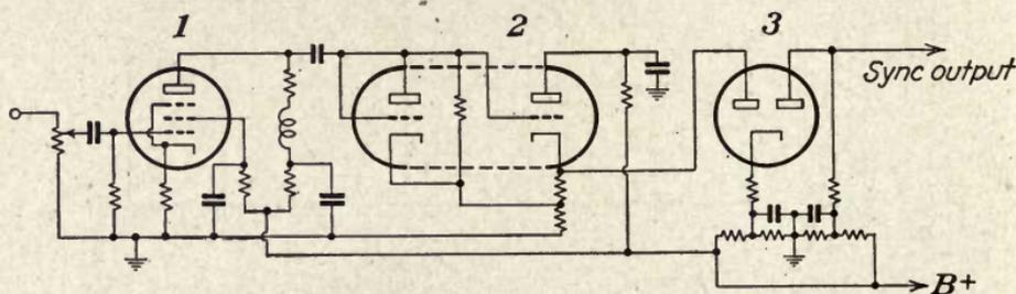
FIG. 85.—Synchronizing separator circuit. (Campbell and Lempert.)
