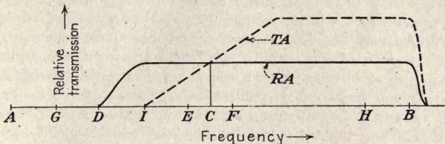
FIG. 26.—Comparison of RA and TA systems, showing transmitter characteristics in the two cases. (S. W. Seeley.)
