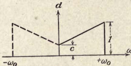
FIG. 34.—Admittance characteristic of a predistorting filter with linearly sloping top. The admittance increases from the value  $c$  at zero frequency to unity at  $\omega_0$ . The phase characteristic is uniform,  $\phi(\omega) = k\omega$ .
