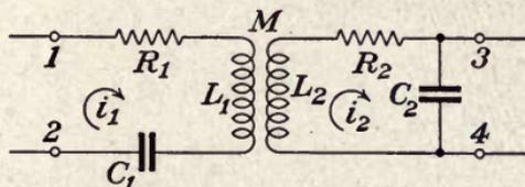
FIG. 99.—Identical series-tuned primary and secondary, constant d-c voltage applied to primary. (G. R. Town.)
