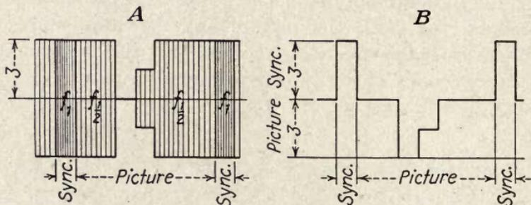
FIG. 68.—Transmitter-output waveforms, method 3. (R. D. Kell.)
