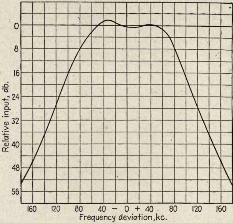
FIG. 15.—Sound-channel bandpass characteristic to limiter grid, receiver X-563.
