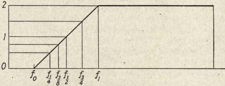
FIG. 65.—Idealized receiver-frequency characteristic. (R. D. Kell.)
