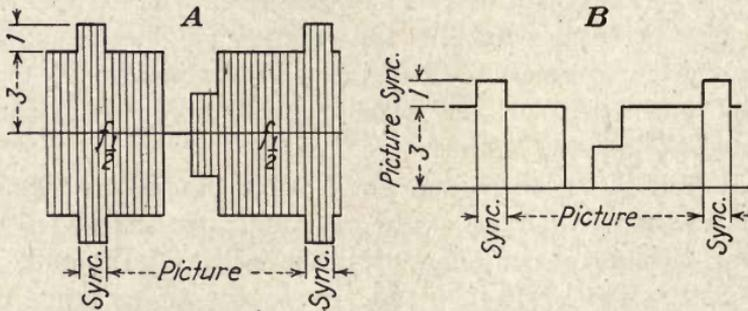
FIG. 66.—Transmitter-output waveforms, method 1. (R. D. Kell.)
