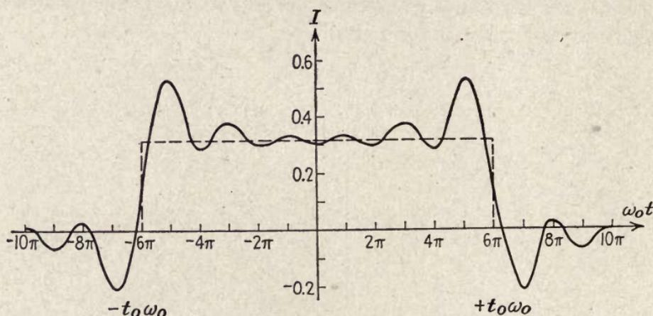
FIG. 37.—Response of the filter of Fig. 34 to the square pulse, for  $c = 0.5$  and  $\phi = 0$ . The peak-to-peak amplitude is 0.735. The signal to noise gain at the top frequency is 4 db, whereas the loss at zero frequency is 6 db.
