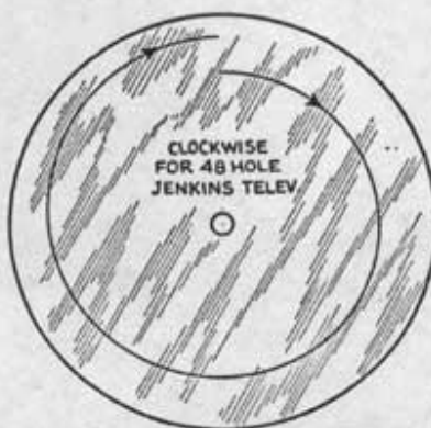
Direction of rotation of disc necessary to receive the images broadcasted by the Jenkins Television transmitting station.
