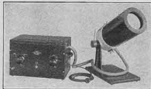
A portable cathode-ray oscilloscope with power supply. The potentiometer at the left controls the potential on the anode, to make the tube more brilliant (right) or more sensitive (left). The right-hand knob controls the focussing field
