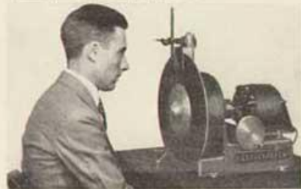
MECHANICAL details of the television receiver. Viewed through the aperture of the metal plate, the holes in the disc form moving spots of varying brightness which paint a picture on the retina of the eye.
