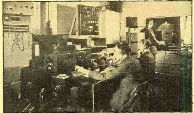
CONTROL ROOM OF THE BBC STATION This is the control room of the television studio with the sound-control engineer, at left, and a visual-control engineer on his right.
