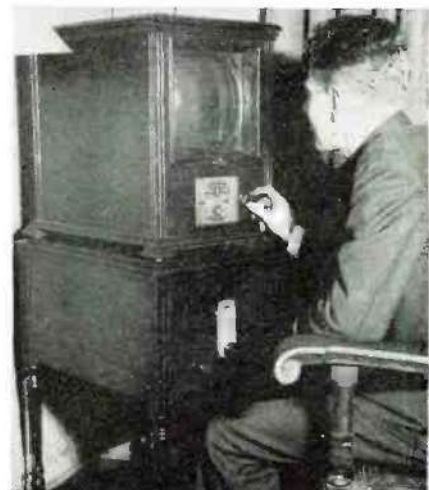
Home tele-receiver of 1930 with its huge magnifying glass and scanner.
