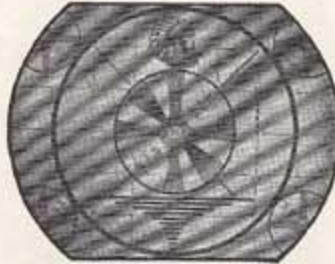
Figure 12. Short wave transmitter interference.
