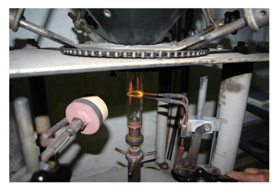
You want the flames to hit both sections of glass equally, so they heat up at the same rate. If the flame heats one section more than the other, the result will be a bad joint because one piece was cooler than the other. After a few seconds the glass will be at the correct temperature, and the lower chuck should be slowly raised so the 2 pieces meet plus an additional 1mm or so to allow the glass to 'mix'.
