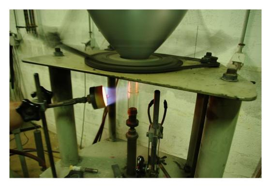
Reduce heat applied to the glass by progressively pulling the burner away over a period of 3 minutes. After that, the flame may be extinguished. The glass will still be quite hot at this point, and subject to thermal shock if it comes into contact with overly cool air or liquids. Therefore the tube should be placed in an environment with as little moving air as possible, and allowed to cool to room temperature on its own.
