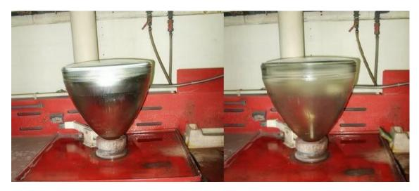
The chemical screening recipe for each tube depends on the size of the bulb and type of phosphor, different mixtures are calculated from the master list for odd sizes. In general the mixture in the tube will contain silicate, phosphor, barium oxide and demineralized water.
