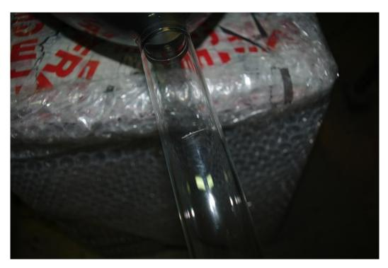
Next position the hot wire around the neck in line with the score in the glass, being mindful that the tips of the tool are to be on either side of the scored line. Turn on the tool, and allow it to heat up. You will hear the glass fracture after about 10-15 seconds, at which point you should remove power from the tool and allow it to cool. The neck should now be fractured all the way around, and you can remove the tool from the neck.
