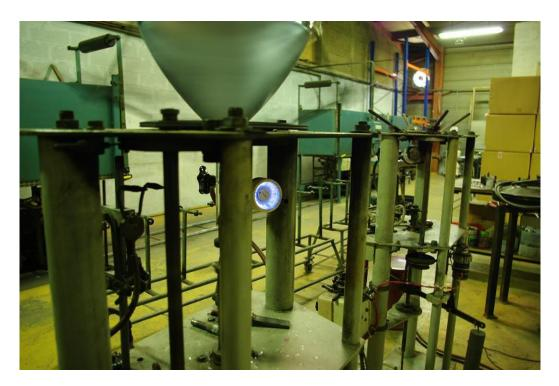
Adjust both gas and shop air supply for a <sup>3</sup>/<sub>4</sub>" protrusion of the flame from the front face of the burner, and allow it to warm up. Once the burner has achieved a nice red appearance on the inside ceramic insulator, the burner is ready.
