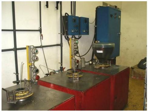
Next lacquer is sprayed for 1 second at low pressure at the tube face, rotating at 90 RPM, running down towards the neck. The tube continues to rotate after spraying for a couple of minutes, to ensure an even coating.
