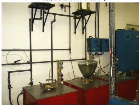
The lacquer is 'cut' with a water jet for several minutes at a predetermined point below the phosphor coating, which removes excess lacquer so the aluminum can bond properly with the glass during aluminization.
