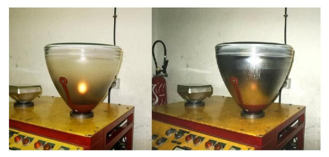
After the coating has been applied, the tube goes into the oven at 410\*C to bake out the remaining lacquer. There is now a thin coating of phosphor and aluminum on the bulb face, separated by the space formerly taken up by the lacquer. A picture tube layer cake! After baking out the lacquer, blow out the fumes on the drying rack. Tube is now gun ready.
