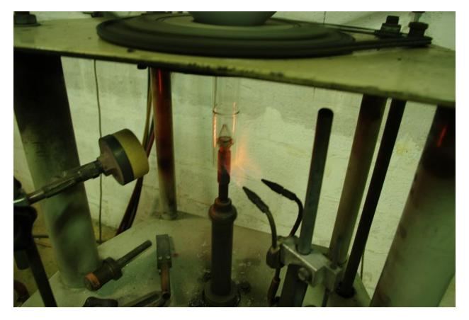
Once the black ring appears around the neck glass, add oxygen to the flame and move in on the button. Positioning of the flame is critical, it should be pointing at the upper edge of the button. If you aim too high, the glass will stretch out too much as it falls, making the joint weak and prone to cracking. Aim too low and the glass won't even touch the button when it falls, then you'll have no choice but to affix a new section of glass and try again.
