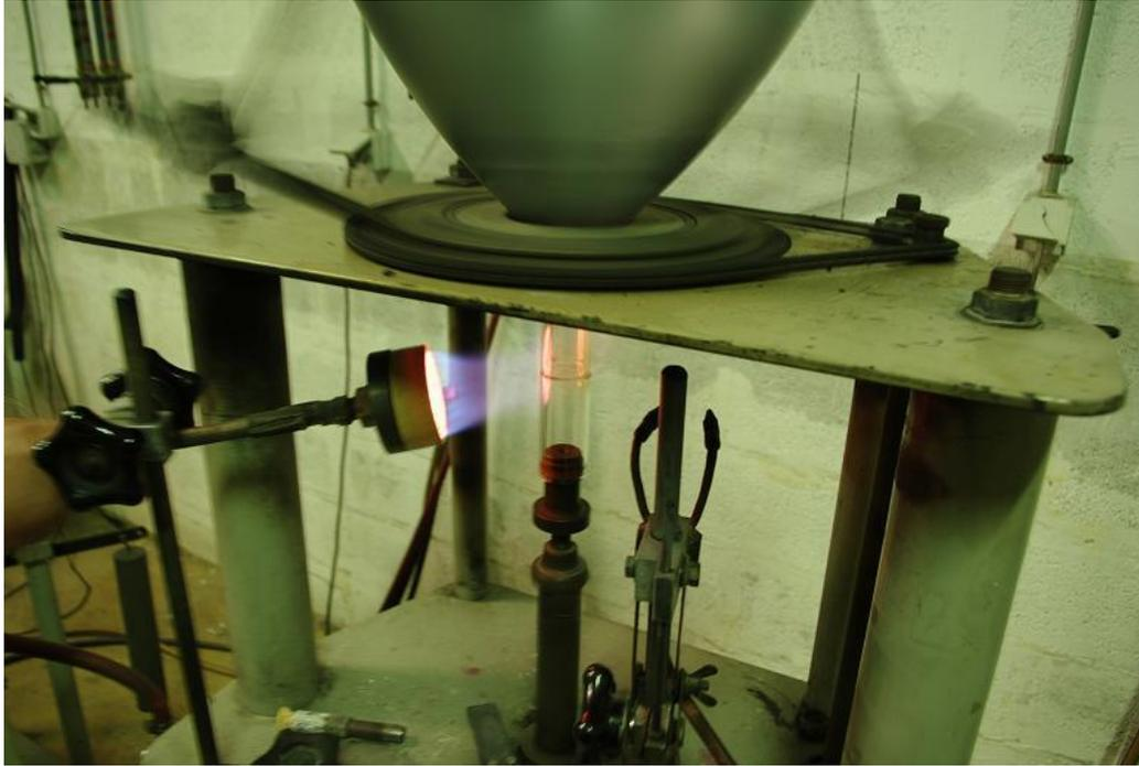
Reduce heat applied to the glass by progressively pulling the burner away over a period of 3 minutes. After that, the flame may be extinguished. The glass will still be quite hot at this point, and subject to thermal shock if it comes into contact with overly cool air or liquids. Therefore the tube should be placed in an environment with as little moving air as possible, and allowed to cool to room temperature on its own.
