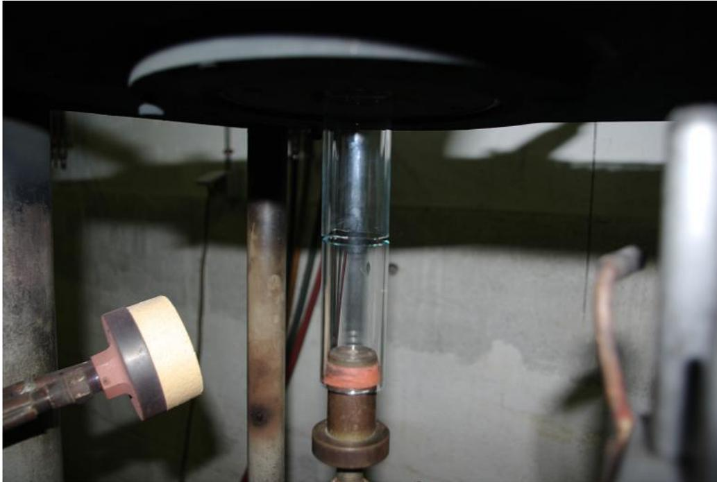
Turn on the natural gas burner, keeping it at distance from the glass for the time being.
