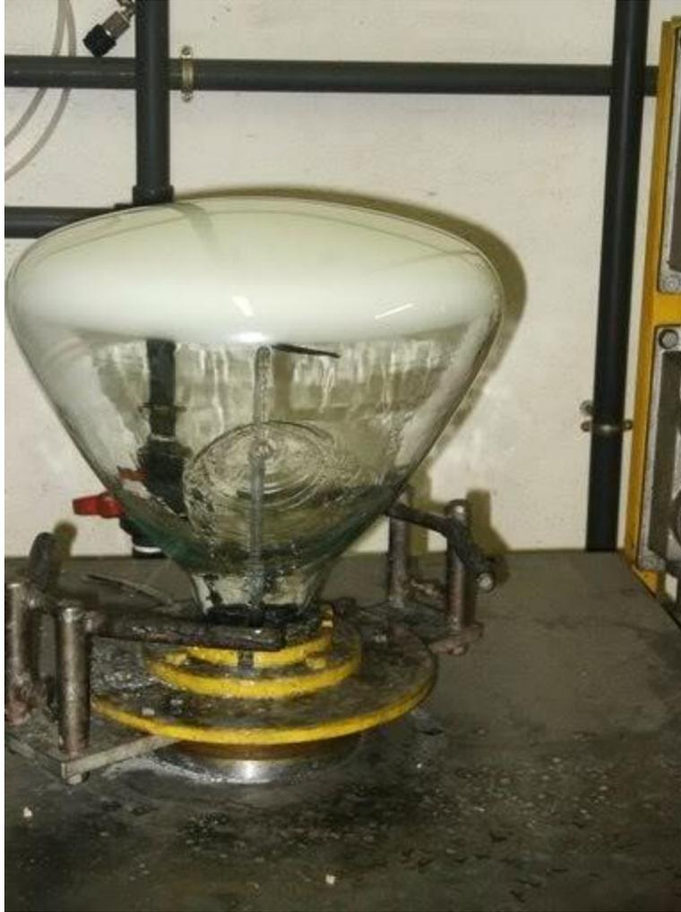
The tube is again sent to the drying rack to remove moisture- there is now a thin coating of lacquer and phosphor, separated by the space formerly occupied by the removed water.
