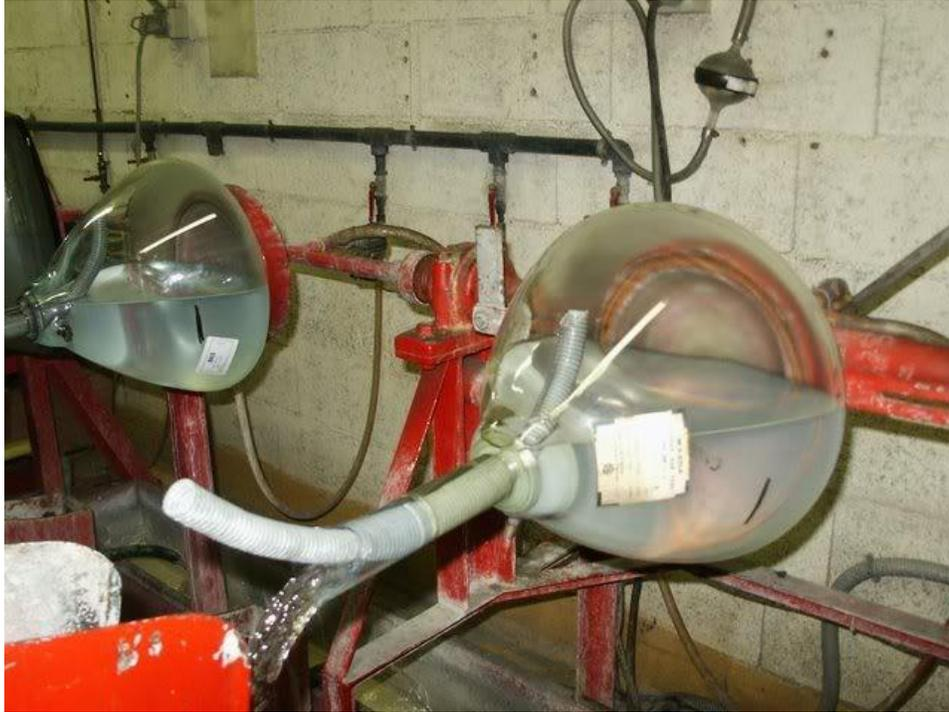
After all the fluid has left the tube, the excess silicate must be 'cut' away from the lower portion of the bulb with a water jet.
