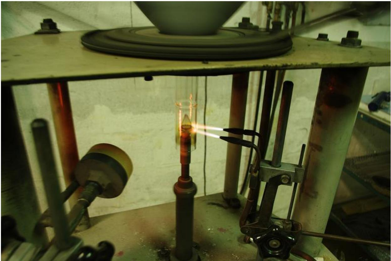
When you notice that the glass has started to melt, follow it on its downward path with the flame. You want to stop it from falling with the graphite paddle, about 1-2" of fall is appropriate.
