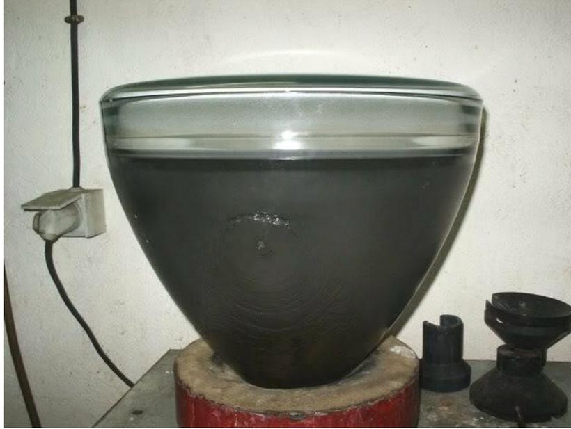
Then it is placed on a heated air drying rack, so the coating can solidify and attach itself properly to the tube face.
