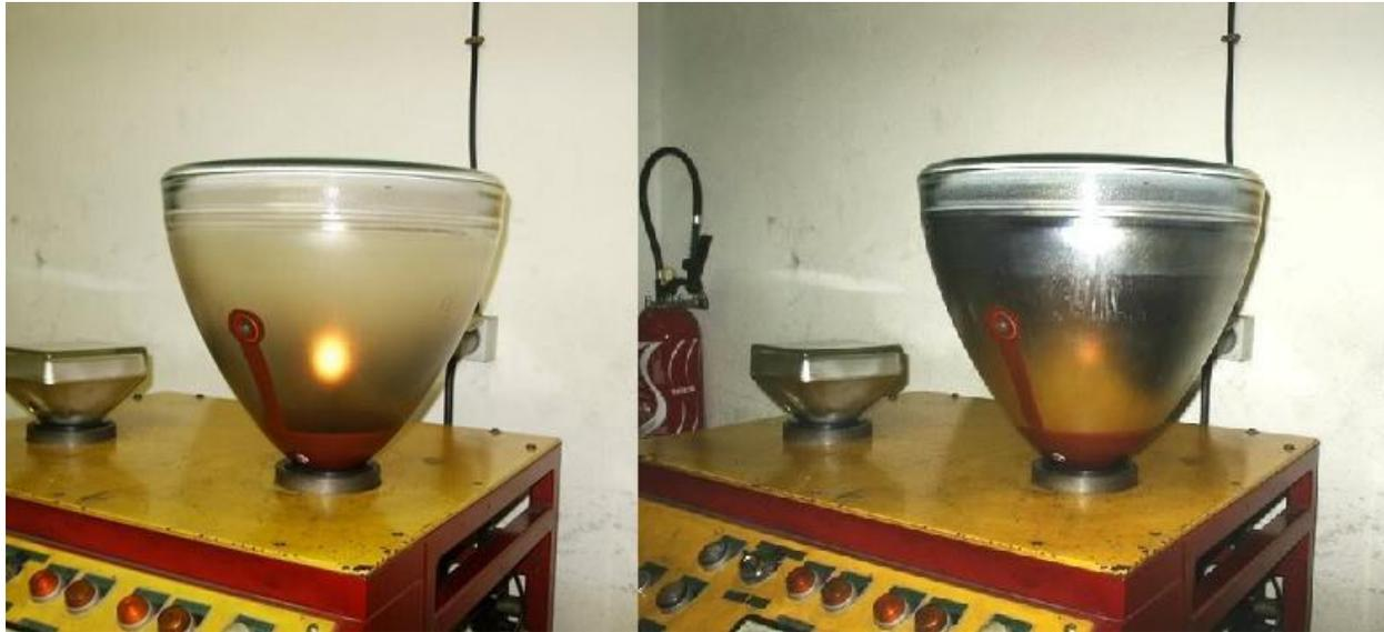
After the coating has been applied, the tube goes into the oven at 410°C to bake out the remaining lacquer. There is now a thin coating of phosphor and aluminum on the bulb face, separated by the space formerly taken up by the lacquer. A picture tube layer cake! After
