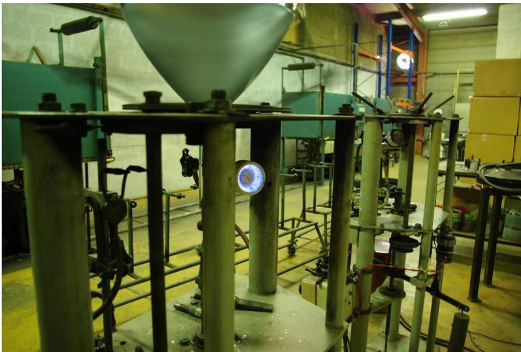
Adjust both gas and shop air supply for a  $\frac{3}{4}$ " protrusion of the flame from the front face of the burner, and allow it to warm up. Once the burner has achieved a nice red appearance on the inside ceramic insulator, the burner is ready.
