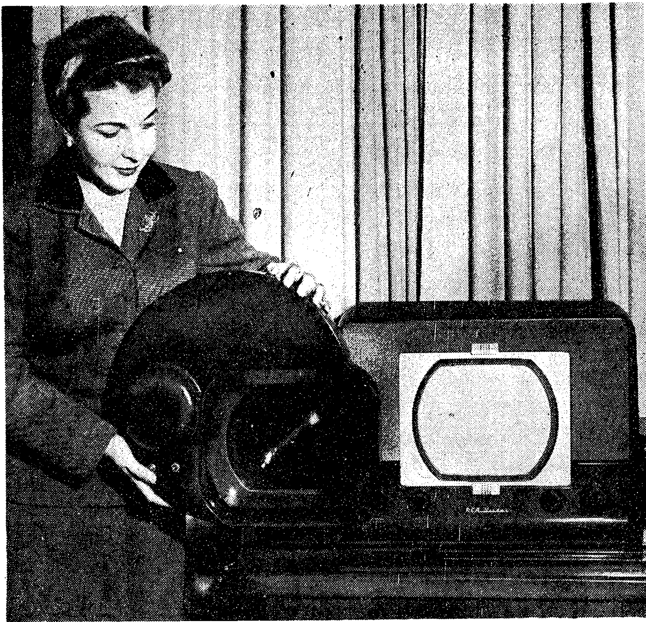
At the Columbia Broadcasting System's offices Margaret Arlen pushes a C. B. S. converter into place in front of the screen to receive picture in color.
