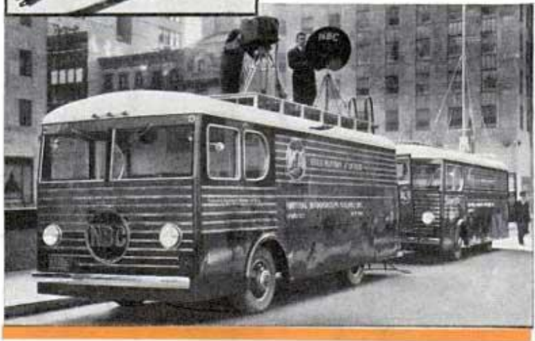
Top, watching television pictures on indirect viewing mirror under lid of receiver, which has twelve-inch kinescope and thirty-six tubes. Center, the kinescope receiving tube and iconoscope, "eye" of transmitter. Below, mobile television station which picks up image and sound in the field
