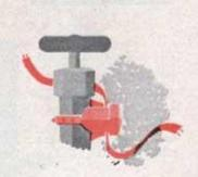
Special television lightning arrester in lead-in wire is required by electric code.
