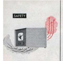
Closely packed components make sets run hot, may cause fire if vents are blocked.
