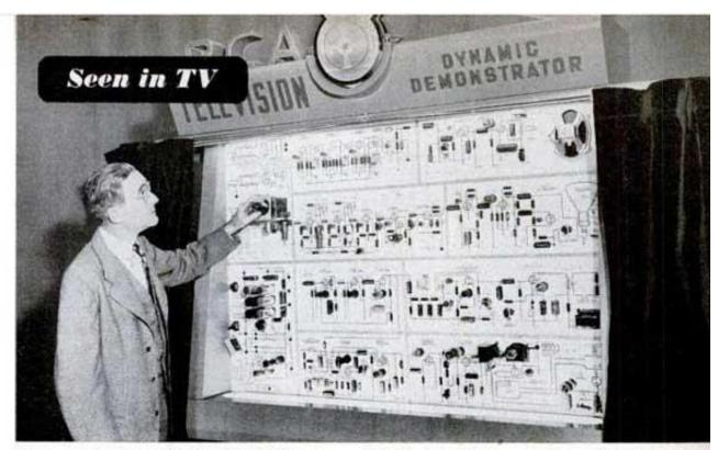
Demonstrator Shows TV IIIs. A complete, working television receiver flattened out on a 3½' by 5½' panel is expected to help servicemen identify and cure many set troubles. The demonstrator above, built by John Meagher, of RCA, is now touring the country. It is used in conjunction with
