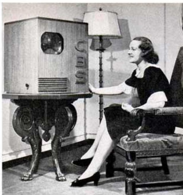
A typical home receiver for television in color. The drawing at the right shows how a whirling disk combines red, green, and blue tints in a single image
