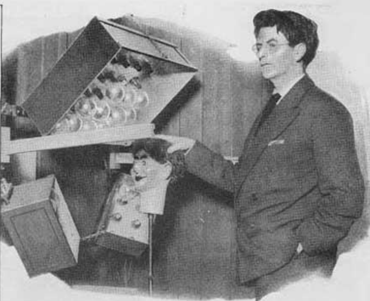
John L. Baird with his sending apparatus in London sending a dummy by television to America just before he sent a living face. Left: Receiving the image, seen in left side of cabinet
