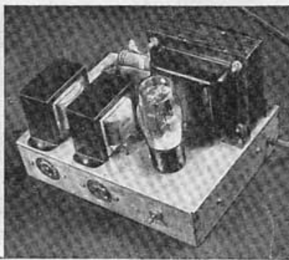
Left—2" C-R tube and Sweep-Oscillator unit; Right—power supply.
