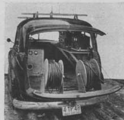
Fig. 4. Rear view of mobile test unit. Cables connect receiving and transmitting antennas to test equipment.
