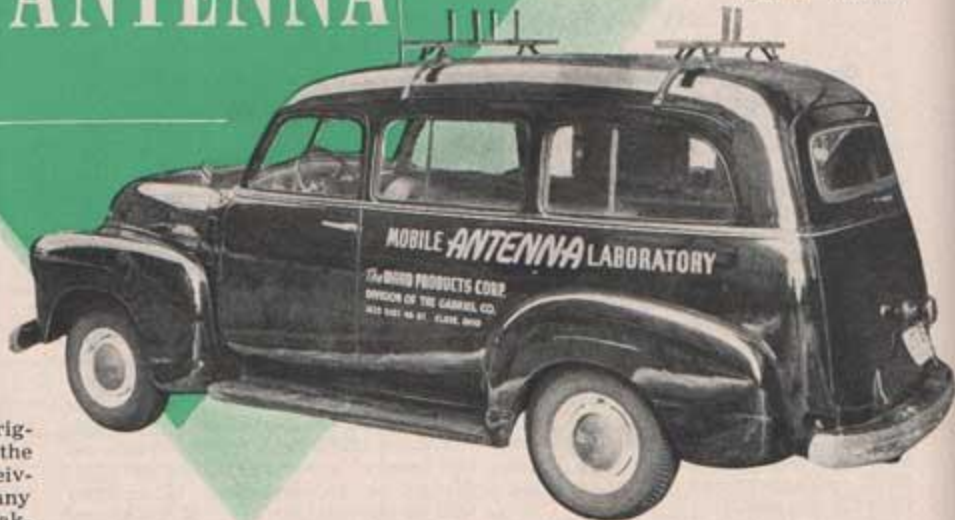
Fig. 1. Test truck completely equipped to make field tests of any type TV antenna.
