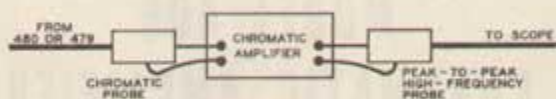
FIG. 1. TEST SET-UP FOR CHECKING FLATNESS OF VIDEO SWEEP OUTPUT FROM THE Chromatic Probe . IN THIS APPLICATION, THE Chromatic Amplifier OPERATES ALSO AS A FILTER.
